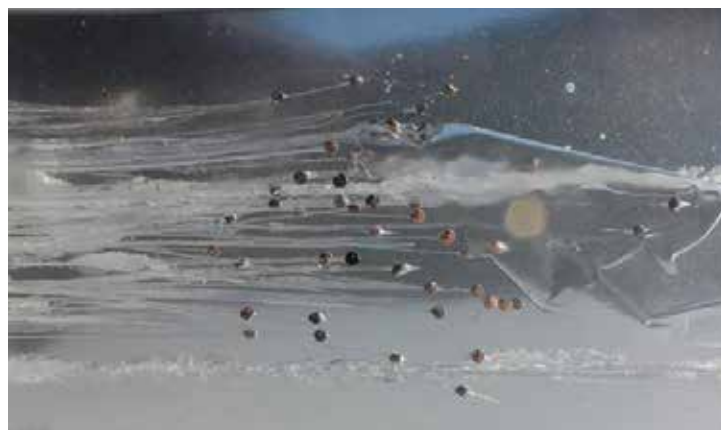
Ballistic gel with 60 pellets of copper-plated #4 birdshot.
